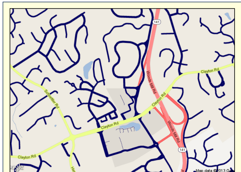
Exhibit 4-11: Map of Chesterfield, Missouri. Neighborhood roads (in dark blue) serve only local residents, directing all traffic to arterial streets (in yellow) where most retail is located. Highways (in red) also serve local travel needs, but carry large volumes of traffic at high speed. Source: © 2013 Google
